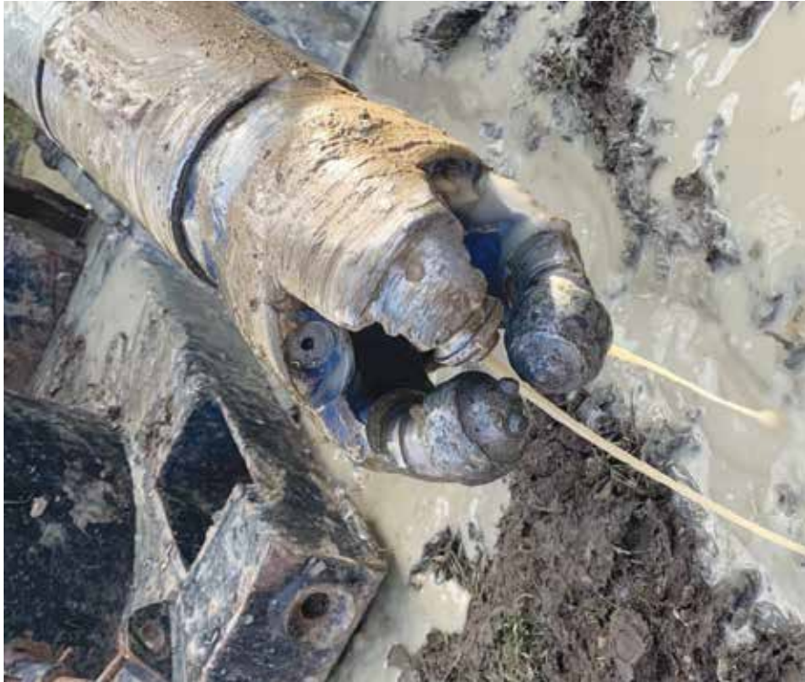
Reduced bit life and inefficiency
