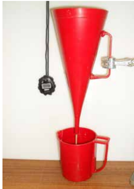
Keep marsh funnel readings between 45 – 75 seconds
