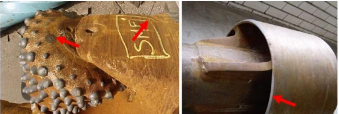
*Examples of tool abrasion resulting from tool gauging*
