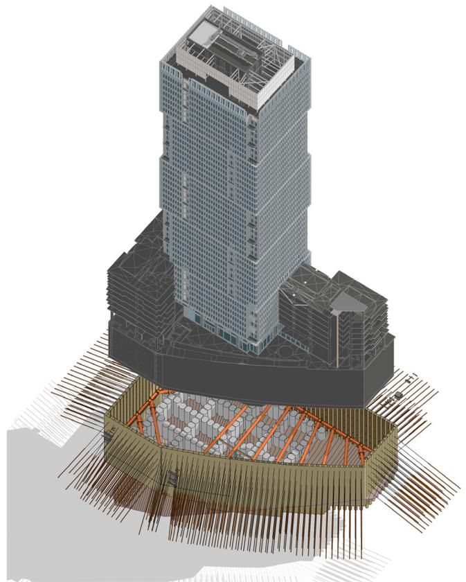
***Transbay Block 9 Support of Excavation: Cutter Soil Mix and soldier pile wall with four levels of tiebacks and one lower level of internal bracing. Brierley also performed the modeling of existing bedrock surface, the jet grouted soil improvement scope and also modeled portions of the existing utilities in the tieback areas to ensure a conflict free design.***
