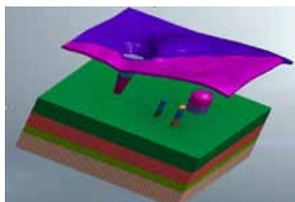
3D FE model for deep strategic gas storage. Parts of the model are removed to expose the storage caverns and the deep pre-existing sinkhole.
